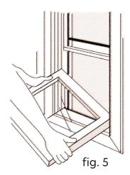
If a balance lock needs to be removed or repositioned, when the sash is removed, a flat head screwdriver can be used to operate the lock and move the balance up and down to position it for pin insertion.
